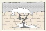
The cavity migrates upward by progressive roof collapse.
